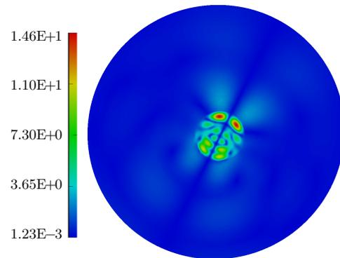
**Fig. 9** Diffraction of an oblique incident SV plane wave by a semi-spherical basin: computed  $y$  component of displacement on basin surface and meshed part of free surface (normalized frequency  $k_S a = 2\pi$ )
