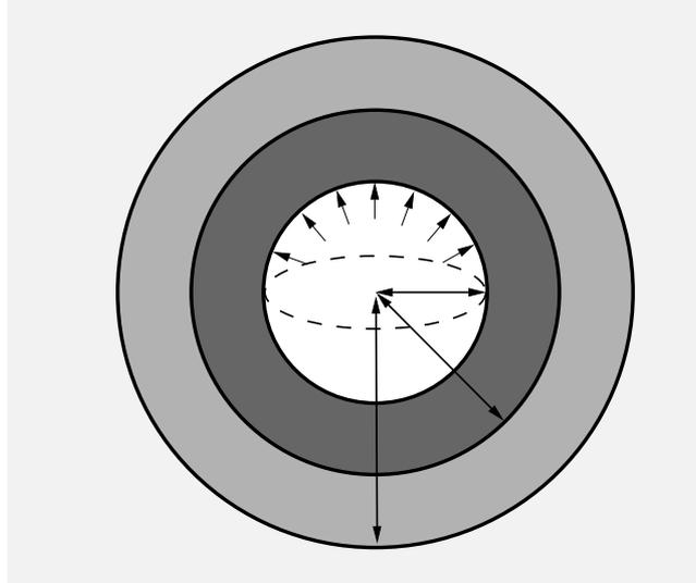
**Fig. 6** Test problem: pressurized spherical cavity surrounded by concentric layers
