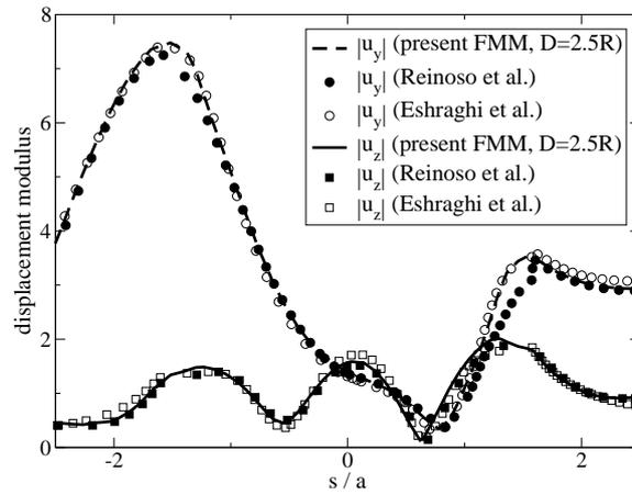
**Fig. 5** Scattering of SV waves by a semi-spherical canyon: horizontal and vertical computed displacement on line ABCDE (with points A, B, C, D, E defined on Fig. 3) plotted against normalized arc-length coordinate  $s/a$  along ABCDE ( $\theta = \pi/6$ ,  $k_S a = 0.75\pi$ )
