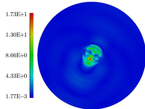
**Fig. 10** Diffraction of an oblique incident SV plane wave by a semi-spherical basin: computed  $z$  component of displacement on basin surface and meshed part of free surface (normalized frequency  $k_S a = 2\pi$ )
