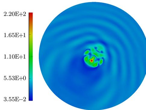
**Fig. 8** Diffraction of an oblique incident SV plane wave by a semi-spherical basin: computed  $x$  component of displacement on basin surface and meshed part of free surface (normalized frequency  $k_S a = 2\pi$ )
