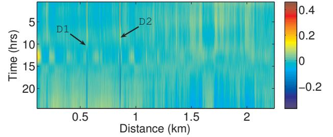
Fig. 5. The residue subspace,  $Y_{residue}^i$ , obtained with SVD for day 1 of nonconsecutive 30 days data set. This subspace represents the deviation from the reference subspace,  $Y_{sig}^i$ , thus putting into evidence the singularities.
