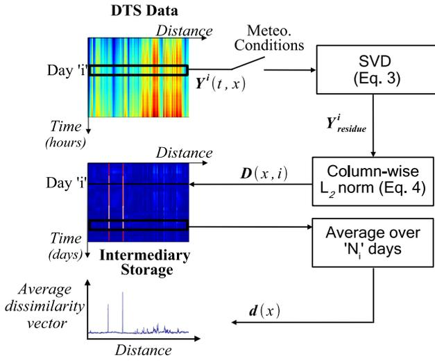
Fig. 4. SVD based singularity detection system.
