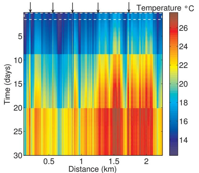
Fig. 2. Real DTS temperature data set for 30 nonconsecutive days, having no precipitation instances, during summer 2005. The color map shows different observed temperatures with increasing temperatures from blue to red.
