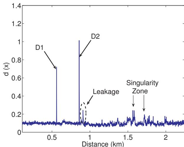
Fig. 9. The dissimilarity measure for temperature data acquired in 2007 reveals occurrence of a real water leakage in 2007.
