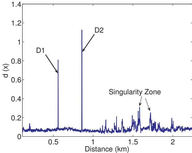
Fig. 7. The average dissimilarity vector for spring 2006 validates the repeatability of the proposed system by detection of the drains and singularity of the ground surface as major singularities.
