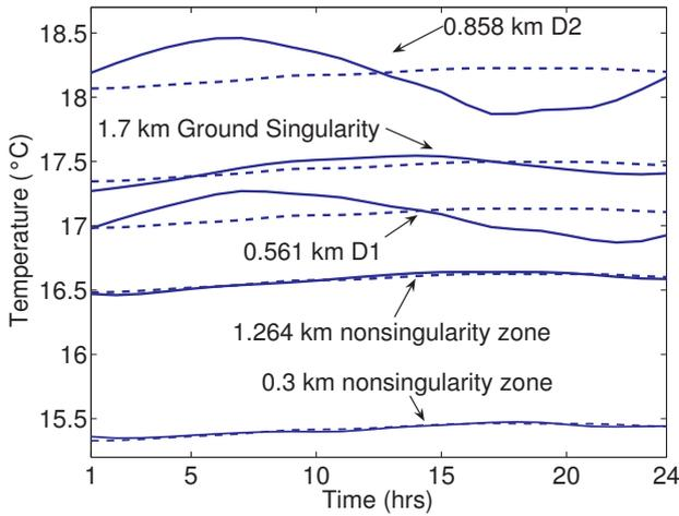
Fig. 3. (Solid Lines): The 24-hour temperature profiles on day 1 at 5 different distances of image in Fig. 2 (see white rectangle and arrows). The singular zones ( $D1$ ,  $D2$  and 1.7 km) present a different trend as compared to nonsingular zones (0.3 km and 1.264 km). (Dashed Lines):  $\mathbf{Y}_{sig}^1$  at same day and distances as solid lines, showing that estimated reference vectors for singular zones have large deviations as compared to nonsingular zones.
