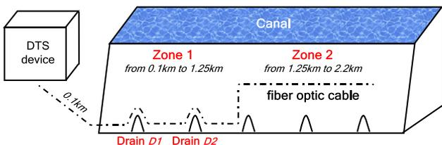
Fig. 1. The configuration of data acquisition at the experimental site.
