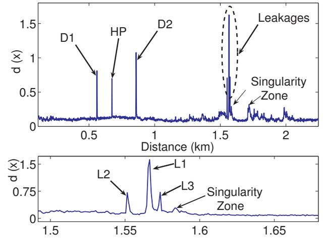
Fig. 8. (Top): The mean dissimilarity measure in case of artificial leakages show the detection of the 3 leakages and the hot point,  $HP$ , in addition to permanent singularities,  $D1$ ,  $D2$  and ground singularity zone. (Bottom): The zoomed view in the vicinity of artificial leakages shows leakage  $L1$  offering the most dissimilarity due to its highest flow rate.
