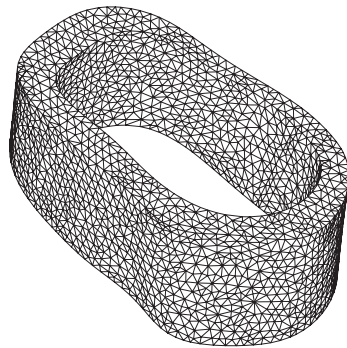
Figure 5: CAD numerical model and mesh of the first bone sample performed with about 30,000 tetrahedral elements.
