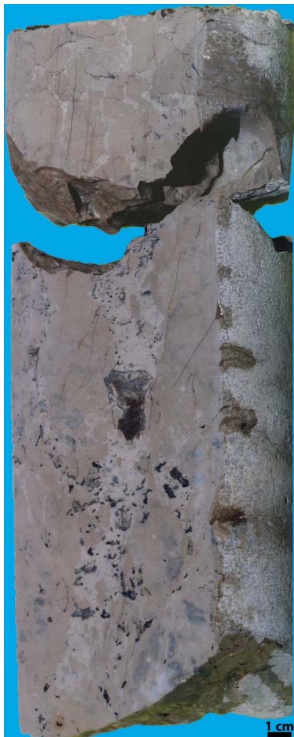
Figure 2: A set of 2 core slabs illustrating karstic features.- Bu Haseer regional Substage, well N° ZQ of field 'X', offshore Abu Dhabi.
