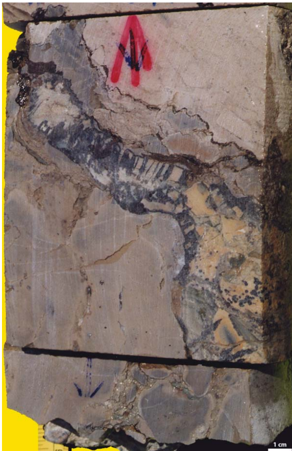
Figure 16: A set of 3 core slabs illustrating karstic features at the Bu Haseer - Belbazem boundary, well N° IFI of field 'X', offshore Abu Dhabi. The facies above the bedding-parallel stylolitic joint consists of lithoclastic rud- to float- stones with a packstone matrix.
