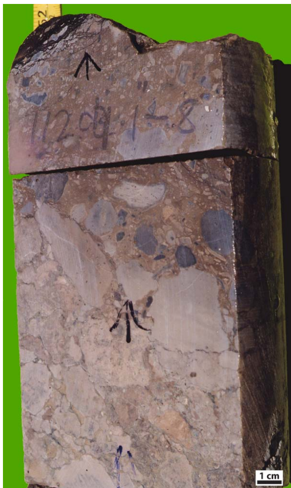
Figure 4: A set of 2 core slabs illustrating the transition from karstic features to lag deposits (floatstone of extraclasts with a wacke- to pack- stone matrix).- Bu Haseer regional Substage, well N° IFI of field 'X', offshore Abu Dhabi.
