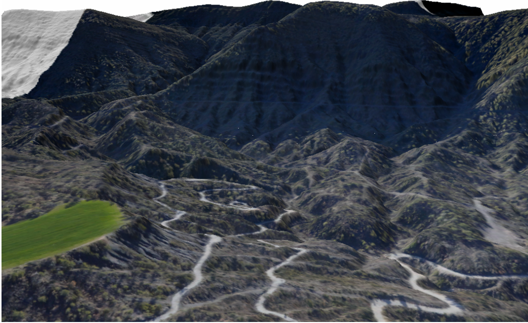
Fig. 11. 3D bird's eye view of the textured DTM over Le Brusquet, France. The texture image is the orthorectified image.
