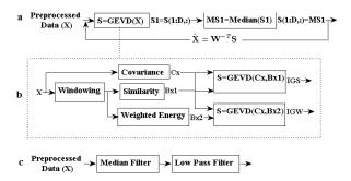
Figure 3: Flowchart of proposed MR artifact reduction algorithms. (a) Iterative GEVD; (b) IGS and IGW, and (c) Median-low-pass filtering. D is the number of first few components in which the MR artifact is most amplified.
