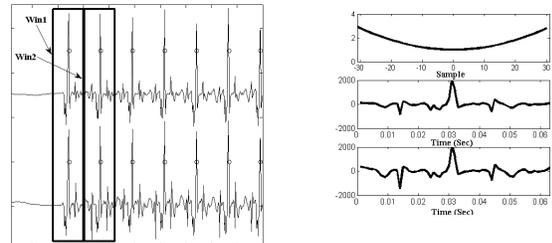
Figure 1: Peak detection and windowing on MR artifact of EEG signal. Peaks are shown with circles.
