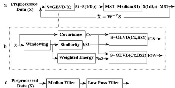
Figure 3: Flowchart of proposed MR artifact reduction algorithms. (a) Iterative GEVD; (b) IGS and IGW, and (c) Median-low-pass filtering.  $D$  is the number of first few components in which the MR artifact is most amplified.
