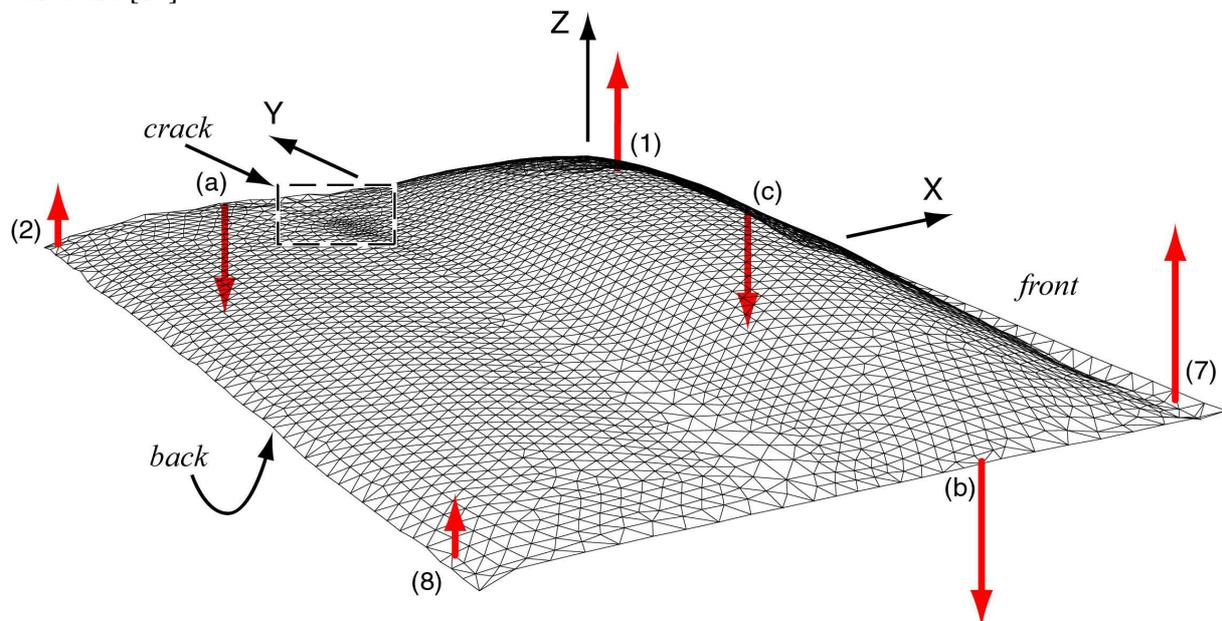
Fig. 3 Finite elements mesh of the panel and applied boundary conditions.
