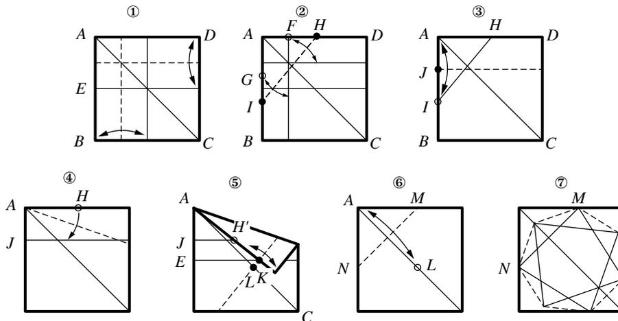
Figure 11: Folding sequence of the optimal heptagon
