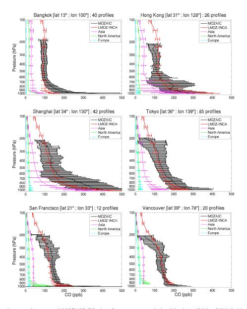
**Fig. 2.** Comparison between the averaged MOZAIC CO aircraft measurements during March-April-May 2005 (in black) and the corresponding LMDz-INCA simulation (in red) above 4 cities in Asia and 2 in western America. The regional contributions to the model CO are also plotted (contribution from Asia corresponds to the sum of all regions in Fig. 1), as well as the standard deviation of the measured and modeled mixing ratios during the time period.
