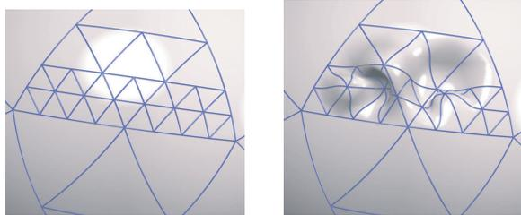
**Figure 1. Left: Locally refined  $G^1$  continuous surface. T-junctions of the parameter domain may occur. Thus coarse patches may be adjacent to several finer patches. Right: Degrees of freedom of the refined patches serve to fit finer details.**
