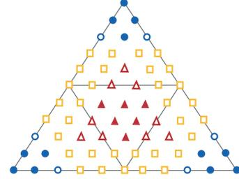
**Figure 4. Control points of a macro-patch which is composed of four quintic Bézier triangles. The control points symbolized by circles are dealt with by step (S1). Squared control points are computed by steps (S2) and (S3). Step (S4) involves the control points symbolized by triangles.**
