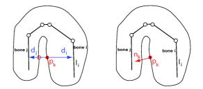
Figure 5: When computing skinning weights, we avoid influence of skin parts which are geometrically close, but which belong to separated parts. Left: Ray-Tracing and intersection detection is one possibility. Right: Test of normal direction compared to the ray is another possibility.
