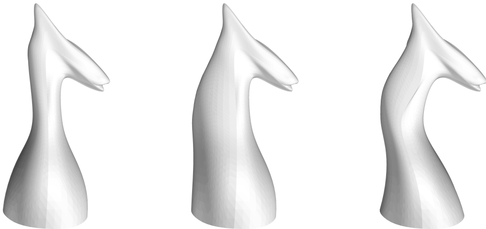
Figure 5: Deformation of a non-uniform B-spline surface. Left: Initial surface. Middle: The volume is free. Right: The volume is preserved.
