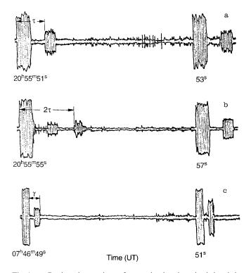
**Fig. 1a–c.** Registration sessions of transmitted and received signals in St. Petersburg: **a,b** guiding waves through the magnetosphere (there and back) with both time-delay  $\tau = 295$  ms and  $2\tau = 590$  ms; 16 November 1985; f = 1.8 MHz; **c** round-the-world propagation via the ionosphere with time-delay  $\gamma = 138$  ms; 22 December 1985; f = 14.1 MHz
