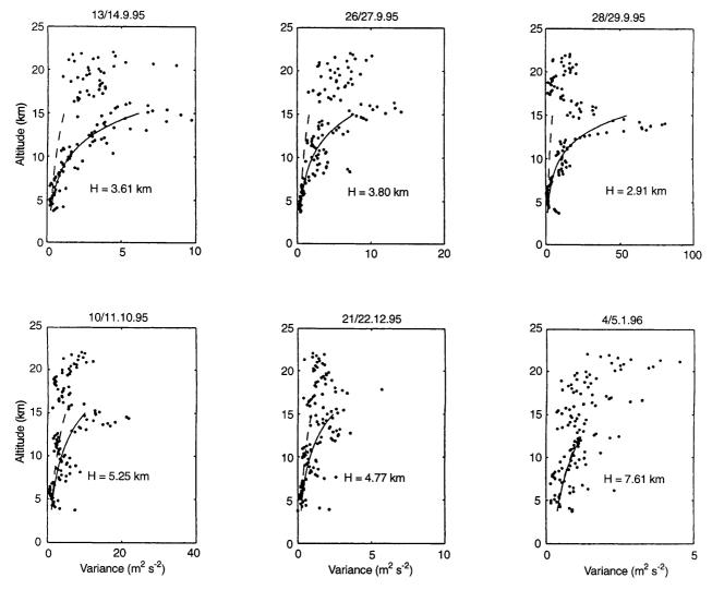
Fig. 5. Altitude variations of the mean square wind fluctuations (points). The solid lines represent exponential curves fitted by least squares method to the observations. The dashed curves are exponential curves with scale height equal to the neutral density scale height (8 km)
