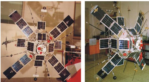
**Fig. 1.** The MAGION-5 flight model assembled and tested in the laboratories of the Institute of Atmospheric Physics, Prague, during winter-spring 1996 and launched on 29 August 1996 as part of the INTERBALL mission. The solar array is shown in the fully deployed position. The MAGION-4 configuration was almost identical.
