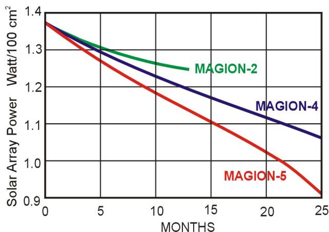
**Fig. 3.** MAGION-4 and MAGION-5 solar array degradation during the 25 months after launch. Most of the differences between these two curves can be explained by the effect of the radiation belts, which is more than 10 times stronger along the orbit of MAGION-5 than MAGION-4. The solar array degradation curve measured on the low-orbiting MAGION-2 (apogee 2400 km) is shown for comparison.
