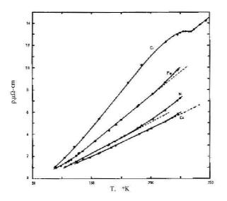
Fig. 5. Resistivity of some transition metals taken from Ref. 24.
