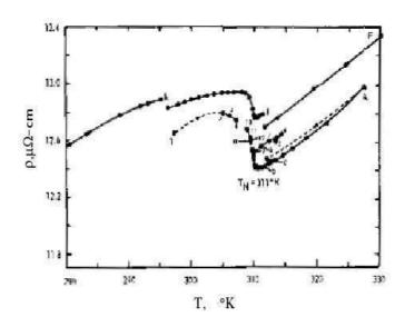
Fig. 6. Resistivity of Cobalt near the Neel temperature  $T_{Neel}$  taken from Ref. 24.
