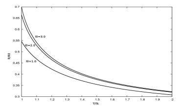
Fig. 12. Normalized resistivity versus temperature for different values of  $l_0$ .
