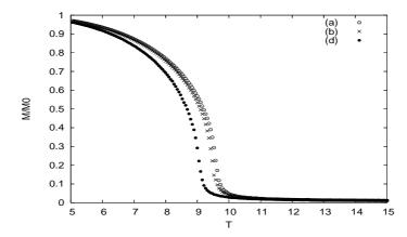
Fig. 24. Lattice magnetization versus temperature T for different concentrations of nonmagnetic impurities: (a)  $C_I = 0\%$  (void circles), (b)  $C_I = 1\%$  (crosses) and (c)  $C_I = 5\%$ (black diamonds).
