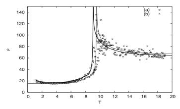
Fig. 26. Resistivity  $\rho$  in arbitrary unit versus temperature T for two cases: without (a) and with 5% of non-magnetic impurities (b) (void circles and crosses, respectively). Our result using the Boltzmann's equation is shown by the continuous curves (see sect. IV): thin and thick lines are for (a) and (b), respectively.
