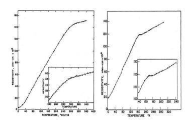
Fig. 2. Resistivity of Gadolinium (right) and Dysprosium (left)taken from Ref. 22.
