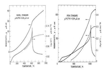
Fig. 4. Resistivity  $\rho(T)$  and its derivative  $d\rho(T)/dT$  obtained for Ni (left) and Fe (right) taken from Ref. 3.
