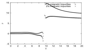
Fig. 30. Resistivity  $\rho_I$  in arbitrary unit versus temperature T. Void circles and black triangles indicate data for 1% and 2% magnetic impurities, respectively.
