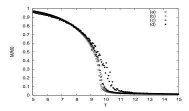
Fig. 20. Lattice magnetization versus temperature T with different concentrations of magnetic impurities  $C_I$ . Void circles, crosses, stars and black diamonds indicate, respectively, data for (a)  $C_I = 0\%$ , (b)  $C_I = 1\%$ , (c)  $C_I = 2\%$  and (d)  $C_I = 5\%$ .
