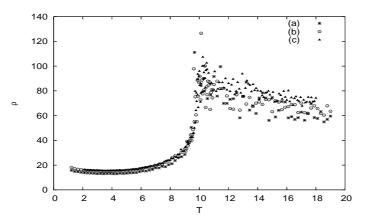
Fig. 16. Resistivity  $\rho$  in arbitrary unit versus temperature T for different film thicknesses. Crosses (a), void circles (b) and black triangles (c) indicate data for bulk,  $N_z=8$  and 5, respectively.
