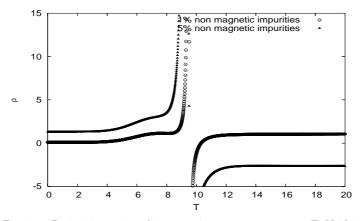
Fig. 31. Resistivity  $\rho_I$  in arbitrary unit versus temperature T. Void circles and black triangles indicate data for 1% and 5% non magnetic impurities, respectively.
