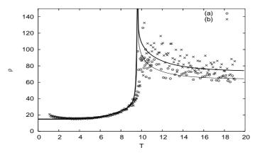
Fig. 22. Resistivity  $\rho$  in arbitrary unit versus temperature T. Two cases are shown: without and with 2% of magnetic impurities (void circles and crosses, respectively). Our result using the Boltzmann's equation is shown by the continuous curves (see sect. IV): thin and thick lines are for (a) and (b), respectively.  $T_c\simeq 9.63$  for 2% .
