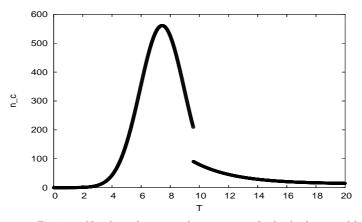
Fig. 29. Number of average cluster size  $n_c$  for both above and below  $T_c$ .
