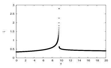
Fig. 28. Mean size  $\xi$  of magnetic clusters versus temperature T for both above and below  $T_c.$
