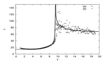
Fig. 25. Resistivity  $\rho$  in arbitrary unit versus temperature *T* for two cases: without (a) and with 1% of non-magnetic impurities (b) (void circles and crosses, respectively). Our result using the Boltzmann's equation is shown by the continuous curves (see sect. IV): thin and thick lines are for (a) and (b), respectively.
