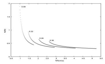
Fig. 13. Normalized resistivity versus temperature for different values of  $\xi$ .
