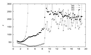
Fig. 19. Resistivity  $\rho$  in arbitrary unit versus T of the system described in the previous figure's caption. Black triangles: resistivity of the surface films, void circles: resistivity of the middle film, black squares: total resistivity. See text for comments.
