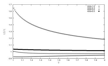
Fig. 9. Relaxation time, Eq. (28a), versus T for different values of  $k_0 d$ .
