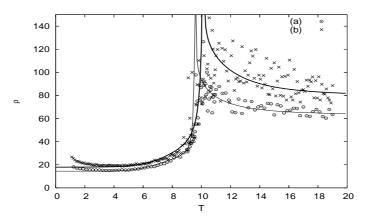
Fig. 23. Resistivity  $\rho$  in arbitrary unit versus temperature *T*. Two cases are shown: without (a) and with 5% of magnetic impurities (b) (void circles and crosses, respectively). Our result using the Boltzmann's equation is shown by the continuous curves (see sect. IV): thin and thick lines are for (a) and (b), respectively.  $T_c \simeq 10.21$  for 5%.
