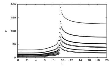
Fig. 32. Resistivity  $\rho$  in arbitrary unit versus temperature T for different densities of itinerants spins. Curves from top to bottom are for  $n_0 = 0.2, 0.33, 0.5, 0.7, 1$  and 1.5.
