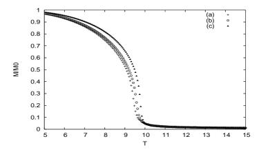
Fig. 15. Lattice magnetization versus temperature T with different thicknesses  $(N_z)$  of the film: crosses, void circles and black triangles indicate data for  $N_z=5$ , 8 and bulk, respectively.  $T_c(bulk) \simeq 9.79$ ,  $T_c(N_z = 8) \simeq 9.58$  and  $T_c(N_z = 5) \simeq 9.47$ .
