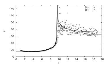
Fig. 21. Resistivity  $\rho$  in arbitrary unit versus temperature T. Two cases are shown: without (a) and with 1% (b) of magnetic impurities (void circles and crosses, respectively). Our result using the Boltzmann's equation is shown by the continuous curves (see sect. IV): thin and thick lines are for (a) and (b), respectively. Note that  $T_c \simeq 9.68$  for  $C_I = 1\%$ .
