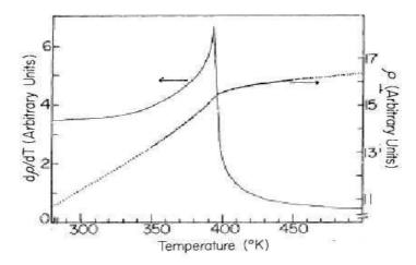
Fig. 3. Resistivity  $\rho(T)$  and its derivative  $d\rho(T)/dT$  for  $GdCo_2$  taken from Ref. 23.
