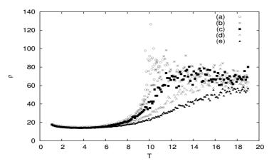
Fig. 17. Resistivity  $\rho$  in arbitrary unit versus temperature T, for different magnetic fields. Void circles, stars, black rectangles, void triangles and black triangles indicate, respectively, data for (a) B = 0,(b) B = 0.1J,(c) B = 0.3J,(d) B = 1J and (e) B = 2J.
