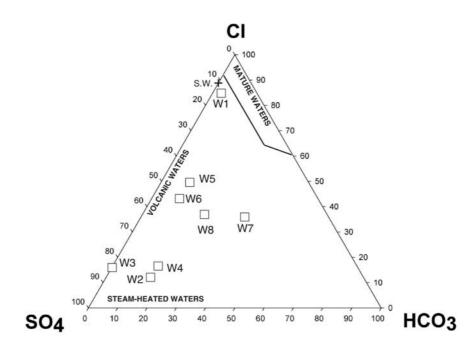
Figure 2. Ternary plot (Cl, SO<sub>4</sub>, HCO<sub>3</sub>) for thermomineral waters of Vulcano Island.
