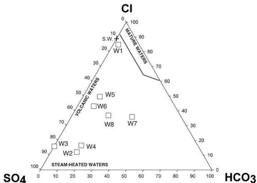
**Figure 2.** Ternary plot (Cl, SO<sub>4</sub>, HCO<sub>3</sub>) for thermomineral waters of Vulcano Island.
