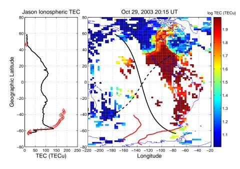
Fig. 3. Whereas the sharp poleward edge of SED, produced by the action of SAPS electric fields, is closely conjugate, the bulge of enhanced TEC at the base of the plume is much more pronounced in the SE U.S. sector.
