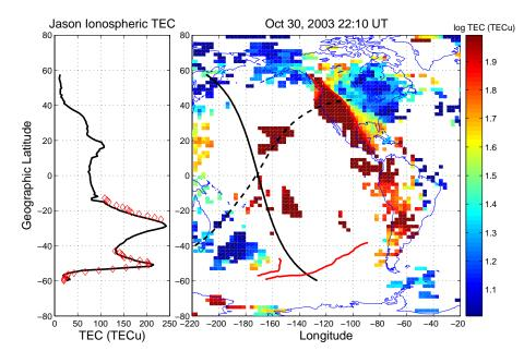
**Fig. 2.** Characteristics of the strong SED plume (>200 TECu) seen over the U.S. mainland and at its magnetic conjugate are similar for the 30 October 2003 superstorm indicating the conjugate actions of magnetospheric electric fields mapping along field lines between hemispheres. The closely-similar magnitude of TEC in the two hemispheres suggests a similar source for the TEC enhancements at low and mid latitudes during that event.
