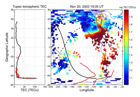
Fig. 4. SED streaming into the polar caps created magnetically-conjugate TOI during the 30 November 2003 event. Topex intersected the southern TOI in the region magnetically conjugate to the GPS TEC SED/TOI observed in the north.
