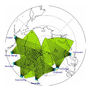
**Fig. 1.** The schematic diagram of the fields-of-view of the Super-DARN radars used in this paper. The inner range interval where the meteor echoes are detected is indicated by the overlapping dark green circles at the beginning of each radar field-of-view.
