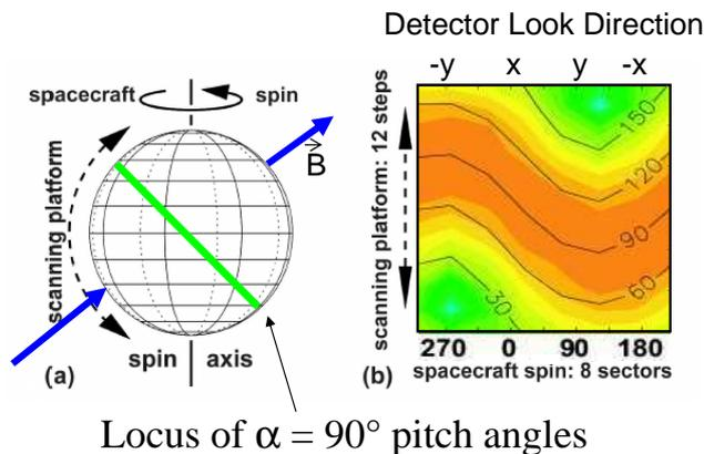
**Fig. 2.** This figure demonstrates how one interprets Figs. 3–5. The detector scans through the unit sphere in 36 s (left) and the fluxes are linearly translated from elevation and azimuth onto an orthogonal Cartesian coordinate system (right). The green line corresponds to the locus of all  $90^\circ$  pitch angles. The blue arrow is the magnetic field vector, where it points from the center of the  $30^\circ$  contour to the center of the  $150^\circ$  contour.
