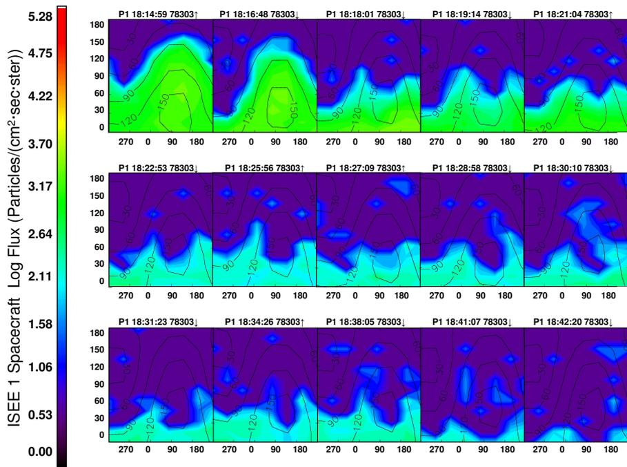
**Fig. 5.** ISEE-1 MEPE 3-D pitch angle distributions for the time period of 18:15–18:42 UT (Epoch 3 in Fig. 1). The s/c has now exited out the “top” of the CDC, but still observes energetic particles from below until 18:42 UT.
