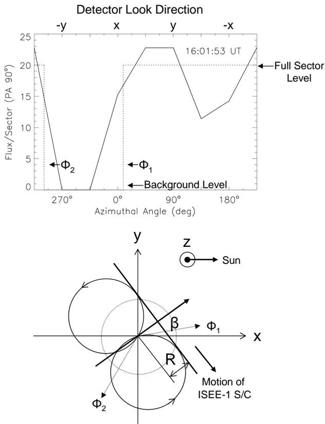
**Fig. 6.** The top plot shows the flux per sector for the 16:01:53 UT record, where there is an absence of particles at a range of azimuthal angles because the s/c is too far away from the CDC boundary to observe particles with those gyroradii. These angles are used to find the orientation angle  $\beta$ , measured from the x-axis, and the distance  $R$  of the boundary from the s/c (bottom). This method is used for Figs. 7–8.
