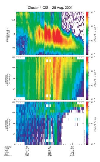
**Fig. 7.** A plot of the CIS data from C4. The top panel is an energyvs-time spectrogram with  $H^+$  energy flux color-coded. The middle and bottom panels display the pitch angle distribution for  $H^+$  and  $O^+$ , respectively.
