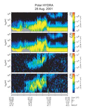
**Fig. 3.** Spectrogram of the Polar HYDRA electron and ion energy flux for the DSIV event of 28 August 2001. Beginning at the top, the panels shown are downward and upward electrons, and downward and upward ions. Inverted-V structures are observed in the interval from about 07:20 UT to 07:30 UT.
