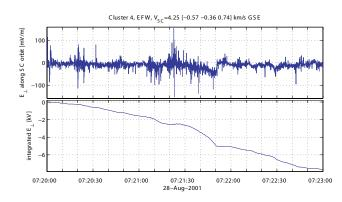
**Fig. 11.** The top panel is the projection of the electric field measured by EFW along the C4 spacecraft trajectory. The data are at a higher resolution than shown in Fig. 10. The second panel is the integral of this electric field along the spacecraft trajectory.
