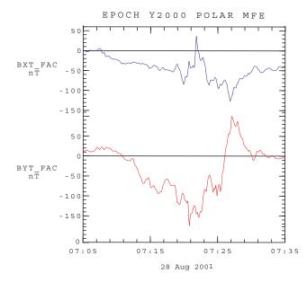
**Fig. 4.** The magnetometer data obtained by the MFE on board the Polar spacecraft for the same time interval. The figure shows  $dB_x$  and  $dB_y$  (perpendicular to ambient magnetic field) in field-aligned coordinates. The characteristic signature of a field-aligned current is observed along with  $f \sim 1/30$  s fluctuations.
