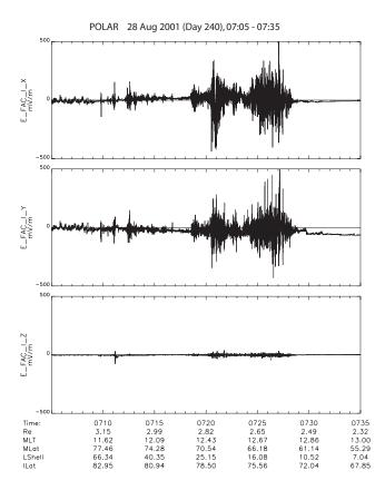
**Fig. 5a.** The presence of a field-aligned current (FAC) is indicated by this electric field data provided by the Polar EFI. In this figure the 3 panels display the x, y, and z components of E with z parallel to B.
