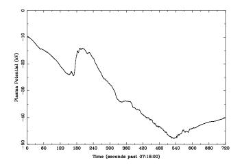
**Fig. 5b.** A plot of the integral of  $\int \mathbf{E} \cdot d\mathbf{L}$  along the Polar spacecraft trajectory. At least three regions of field reversal are seen.
