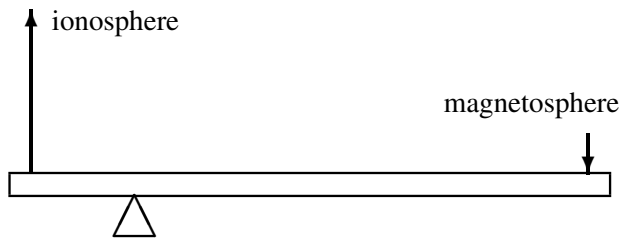
Fig. 2. Relation between forces in ionosphere and magnetosphere for system of region 1 currents (Fig. 1), illustrated by analogy to a simple lever system with mechanical advantage (antisunward is up).
