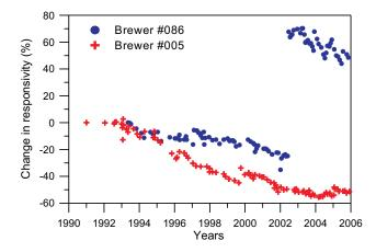
Fig. 2. Time series of the percentage change in the responsivity of the two Brewer spectroradiometers at  $320\pm5$  nm, with respect to the first calibration in their records. The calibration factors have been corrected for temperature effects to a standard temperature of  $25^{\circ}$ C.
