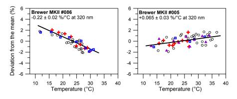
Fig. 5. Percentage deviation of lamp irradiance measurements at 320 nm from their mean, as a function of temperature. Measurements were performed in the laboratory using a 1000 W DXW lamp. The slopes of the regressions represent the temperature coefficients for each instrument, in  $\%/^{\circ}C$ .
