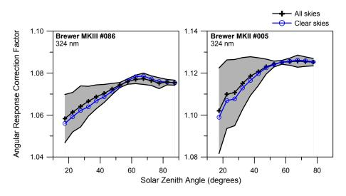
Fig. 4. Average correction factors for the angular response error of the two Brewer spectroradiometers at 324 nm under all skies (crosses) and clear skies (cycles), as a function of solar zenith angle. The shaded area represents the  $1\sigma$  variability for the all-sky average correction factor. The variability of the clear-sky correction factor is very similar and is not shown.
