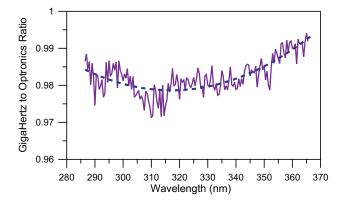
**Fig. 1.** The GigaHertz to Optronics irradiance scale ratio, as determined in 2002, when two new spectral irradiance lamps were obtained from each laboratory. The dashed line is the 2nd degree polynomial fit of the ratio.
