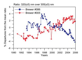
**Fig. 3.** The spectral variation of the calibration factors of Brewers #005 and #086, throughout the period of their operation, expressed by the ratio of the calibration factors at 320 nm ( $\pm$ 5 nm) and 305 nm ( $\pm$ 5 nm).
