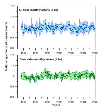
**Fig. 8.** Time series of monthly mean ratios (Brewer #086 over Brewer #005) formed by irradiance integrals (315-320 nm) recorded within 1 min by the two Brewer spectroradiometers at Thessaloniki, under all-sky (upper panel) and clear-sky (lower panel) conditions. The shaded envelope corresponds to the standard deviation  $(\pm 1\sigma)$  of the mean.
