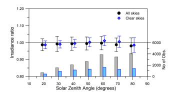
**Fig. 10.** Averages of the ratios (Brewer #086 over Brewer #005) of synchronous irradiance integrals (315-320 nm) recorded by the two Brewer spectroradiometers as a function of solar zenith angle, in intervals of  $10^{\circ}$ , for clear-sky (rhombuses) and all-sky conditions (filled circles). The error bars correspond to one standard deviation.
