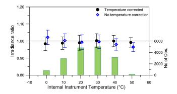
**Fig. 9.** Averages of the ratios (Brewer #086 over Brewer #005) of synchronous irradiance integrals (315-320 nm) recorded by the two Brewer spectroradiometers as a function of the internal instrument temperature, in bins of 10°C. Filled circles correspond to temperature corrected data and rhombuses to data uncorrected for temperature effects. The error bars correspond to one standard deviation.
