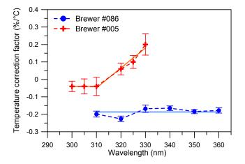
**Fig. 6.** Wavelength dependence of temperature correction factors for the two Brewer spectroradiometers, #005 and #086, derived from linear fits on lamp irradiance measurements conducted in the laboratory in December 2005.
