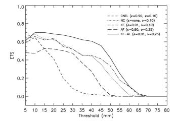
**Fig. 1.** The ETSs of precipitation forecasts in terms of various thresholds (in mm). Curves denote scores for the 6–12 h accumulated rainfall forecasts for experiments CNTL (control run with default values), NC (no convective parameterization), KF (using optimized parameter in the KF scheme), AF (using optimized parameters from both the KF scheme and the Asselin filter).
