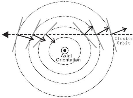
**Fig. 1.** Sketch of the Cluster constellation traversing a 2-D structure. The set of magnetic contour planes are represented by the dashed circles and the normal directions of these planes are the solid arrows. All of these arrows are shown to be perpendicular to the axial orientation of the 2-D structure.
