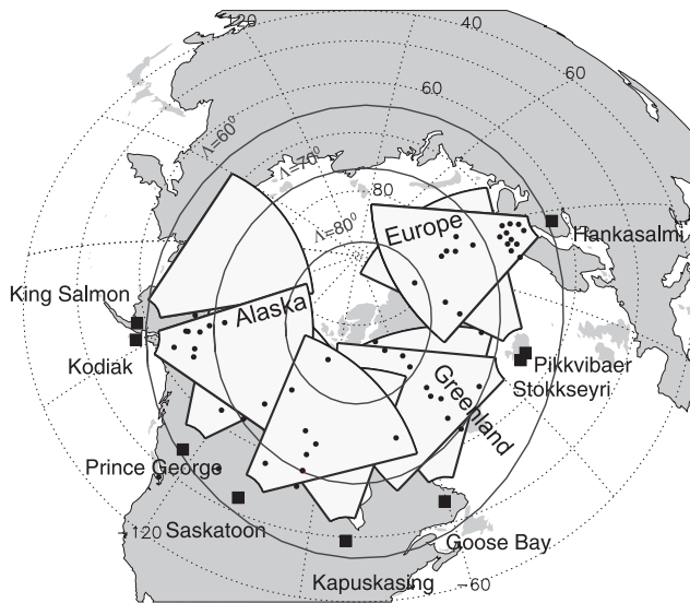
Fig. 1. A map showing the Northern hemisphere SuperDARN radar locations (bold squares), their FoVs (circular sectors), and the magnetometer locations (solid dots). Actual magnetometer data in these sectors (Alaska, Greenland, and Northern Europe) will be presented.
