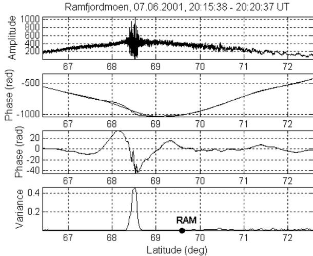
**Fig. 2.** Amplitude (top panel), phase and smoothed phase (second panel from top), phase fluctuations (third panel) and amplitude variance (variance of the logarithmic relative amplitude fluctuations) (bottom panel). The variance averaging interval is 6 s, while the phase is plotted at the 50 Hz-sampling rate of the raw data.
