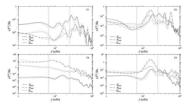
**Fig. 6.** Power spectral densities of the magnetic field components for the interval 18:00 to 18:25 UTC on 21 January 2003. The black curves correspond to the PSD calculated using Welch's method, while the grey curves were obtained using the MEM. The Pi2 band (6.7–25.0 mHz) is enclosed between the vertical dashed lines.
