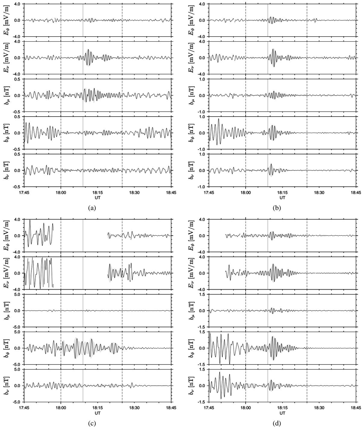
**Fig. 4.** EFW and FGM waveforms for 21 January 2003 on (a) C1 [Rumba], (b) C2 [Salsa], (c) C3 [Samba] and (d) C4 [Tango]. The signals have been bandpass filtered to extract periods in the range 40–150 s. The gaps in the EFW data for C3 and C4 occur where it was not feasible to apply  $E \cdot B = 0$ , and transformation of the electric field to MFA coordinates was thus impossible.
