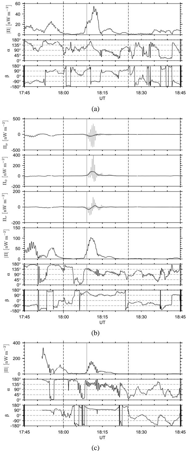
**Fig. 11.** Poynting flux at satellites (a) C1, (b) C2 and (c) C4 during the event on 21 January 2003. In (b) each of the components,  $\Pi_v$ ,  $\Pi_\phi$  and  $\Pi_\mu$ , is filtered over the Pi2 frequency range (grey curve) and averaged over a 150 s window (black curve). The Poynting flux magnitude and orientation angles reflect the 150 s average.
