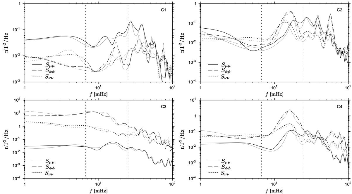
**Fig. 6.** Power spectral densities of the magnetic field components for the interval 18:00 to 18:25 UTC on 21 January 2003. The black curves correspond to the PSD calculated using Welch's method, while the grey curves were obtained using the MEM. The Pi2 band (6.7–25.0 mHz) is enclosed between the vertical dashed lines.
