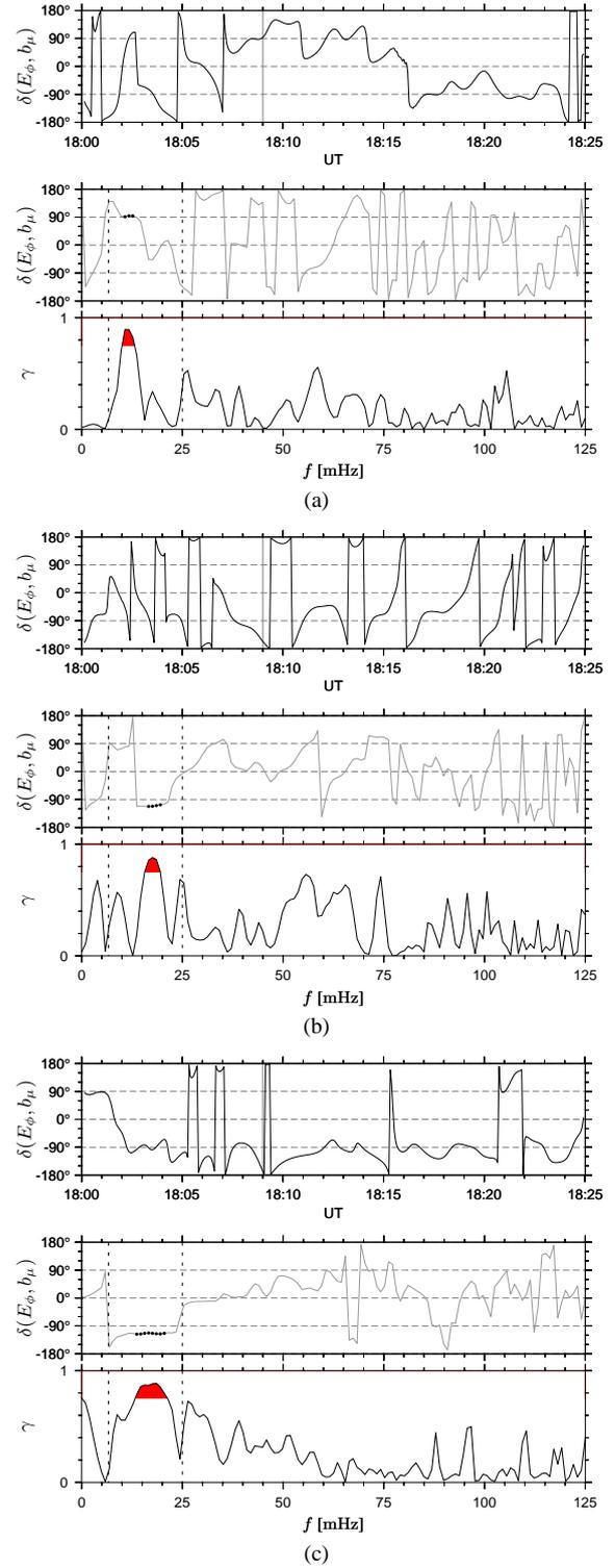
**Fig. 7.** Coherence and phase difference between  $b_\mu$  and  $E_\phi$  at **(a)** C1, **(b)** C2, and **(c)** C4. The shaded portions of the coherence curves indicate frequencies for which  $\gamma$  exceeds the threshold of 75%, and at these frequencies solid points are plotted for the phase difference.
