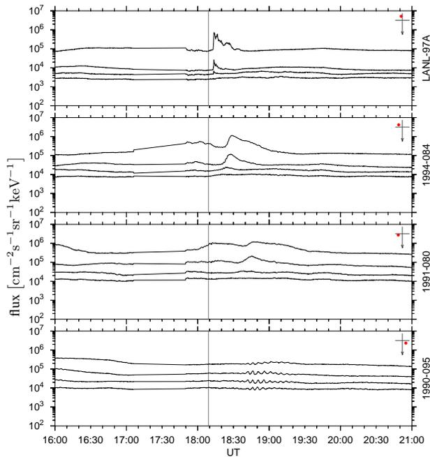
**Fig. 1.** Electron flux data for 21 January 2003 from Synchronous Orbit Particle Analyzer (SOPA) instruments on LANL geosynchronous satellites. The four traces in each panel represent different energy channels; from top to bottom they are 50–75, 75–105, 105–150 and 150–225 keV. In the upper right corner of each panel is an inset indicating the local time of the satellite at the event epoch (the arrow points sunward).
