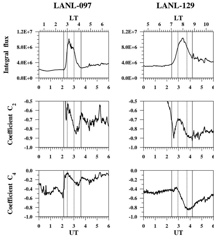
**Fig. 6.** Omnidirectional integral fluxes with energies above 30 keV and the second- ( $C_2$ ) and fourth- ( $C_4$ ) order harmonics of the Legendre polynomial expansion of the pitch-angle distribution function obtained at two geosynchronous satellites.
