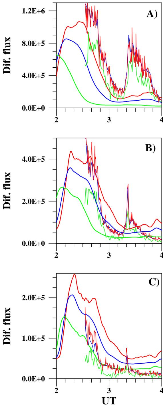
**Fig. 9.** Differential fluxes along (green) and across (red) the magnetic field and omnidirectional fluxes (blue) within the energy channels 21.5–31.5 keV (**A**), 31.5–40.0 keV (**B**), and 40.0–49.5 keV (**C**). The fluxes detected by the CRRES satellite are shown by the thin line. Results of tracing of the fluxes, detected by the LANL-097 satellite to the longitude of the CRRES satellite, are shown by the bold line.
