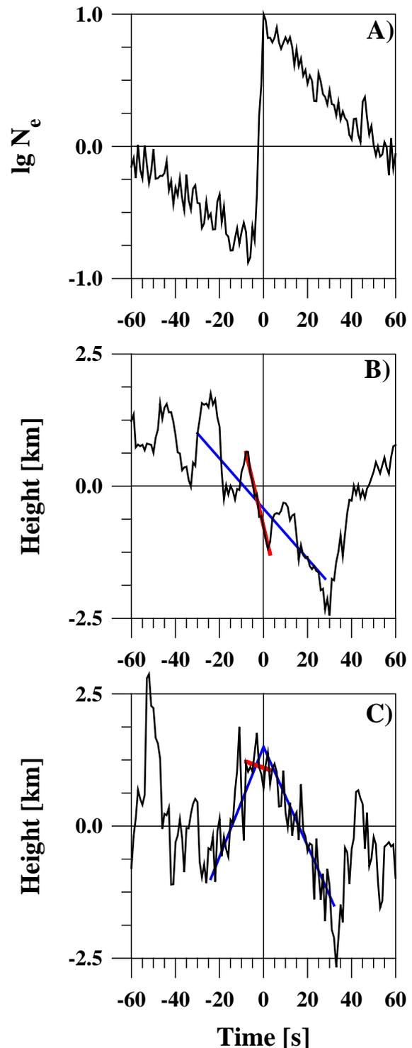
**Fig. 10.** (A) Change in the ionospheric electron density observed by the EISCAT radar during pulsed electron precipitations. (B) and (C) Change in the height of the ionospheric density maximum in the pulses observed in the beginning (B) and at the end (C) of the event.
