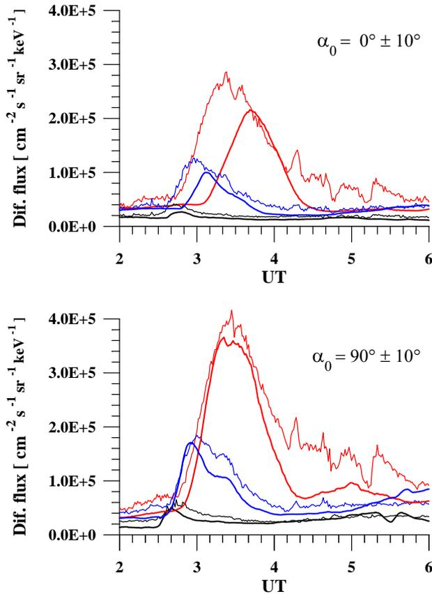
**Fig. 3.** Differential fluxes along (upper plot) and across (bottom plot) the geomagnetic field at 30–45, 45–65, and 65–95 keV (the red, blue, and black line, respectively). The fluxes obtained by the LANL-129 satellite are shown by the thin line. Results of tracing the fluxes, observed by LANL-097, to the longitude of LANL-129 are shown by the bold line.
