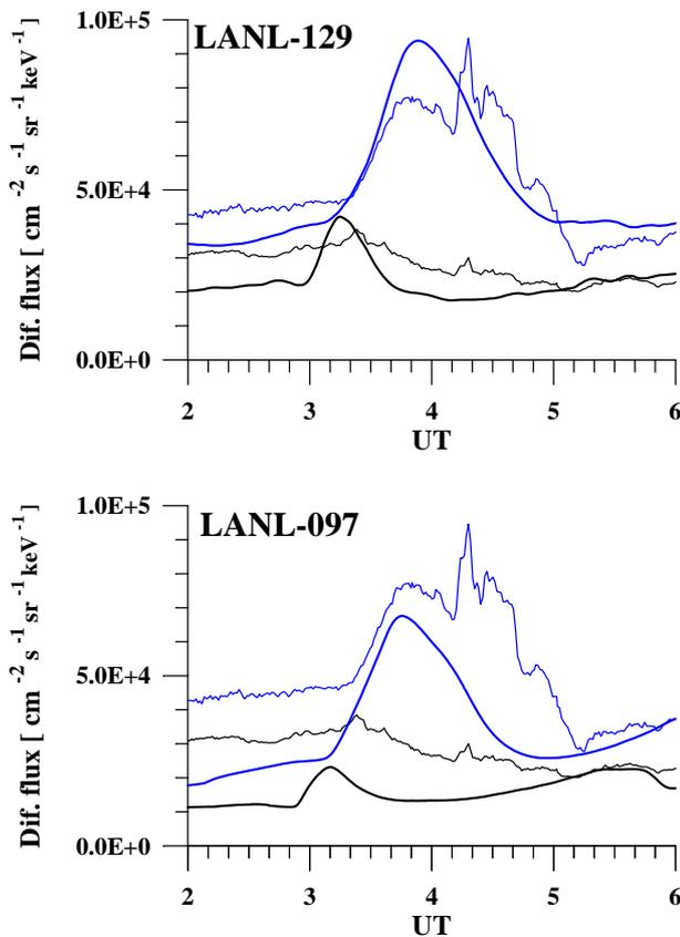
**Fig. 8.** Omnidirectional differential fluxes at 50–75 and 75–105 keV (the blue and black line, respectively). The fluxes obtained onboard the LANL-046 satellite are shown by the thin line. Results of tracing of the fluxes detected by the LANL-129 (top) and LANL-097 (bottom) satellites to the longitude of the LANL-046 satellite are shown by the bold line.
