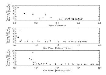
**Fig. 6.** Square difference between observed and best-match predicted phase value (i.e. adjusted for the best phase drift and phase offset) for each data point, as a function of (**a**) recorded coherence of that data point, (**b**) recorded power in the 32-m antenna for that data point and (**c**) associated recorded power in the 42-m antenna.
