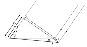
**Fig. A1.** Geometry of observations. *N* is the nominal (horizontal) baseline between the foci of the 42-m and 32-m antennae, *B* is the true baseline and *b* is the vector difference between the two. *s* is a unit vector pointing at the satellite. The true phase path difference is *P*, but that calculated assuming the nominal baseline is  $P_N$ .
