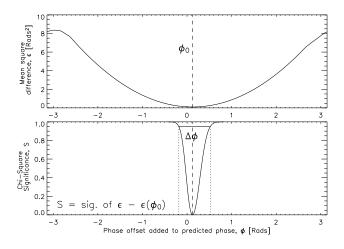
**Fig. 4.** Top panel: Plot of mean square difference between observed and optically-predicted phase values, as a function of phase offset added to the predicted phase. Bottom panel: Plot of significance of the phase offset relative to the best offset found,  $\phi_0$ :  $\Delta \phi$  is the confidence interval in  $\phi_0$  for the 95% level.
