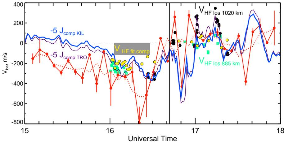
**Fig. 5.** Comparison between the  $E \times B$  plasma drift components as inferred from various techniques. The green squares and black dots (yellow dots) represent the F-region velocity measured by the CUTLASS Finland radar in ranges 870–915 km and 1005–1050 km, respectively (inferred from the cosine fitting to all F-region velocities). The thin dark (heavy) blue line is the reversed equivalent current component at Tromsø (Kilpisjärvi).
