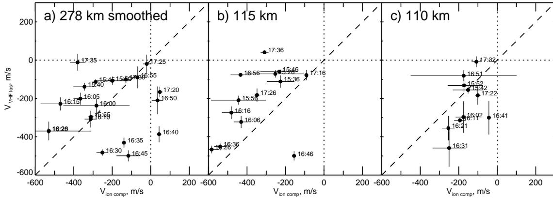
**Fig. 4.** Scatter plots of line-of-sight irregularity drift velocity measured by the STARE Finland radar in beam 4 and bin 24,  $V_{VHF\ los}$ , against the component of the EISCAT ion drift velocity resolved along the STARE beam 4 direction at (a) 278, (b) 115, and (c) 110 km. The time (interval centre) of measurements is indicated near each point.
