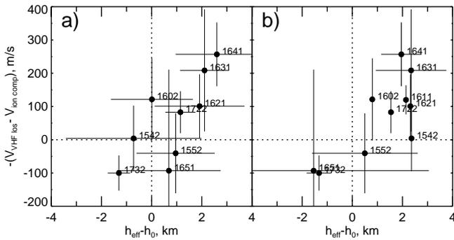
**Fig. 7.** A difference between the STARE l-o-s velocity and the EISCAT ion drift component at 110 km (reversed) versus the effective backscatter height counted from  $h_0=110$  km and averaged for (a)  $\sim 10$ -min intervals centered at the time of the EISCAT measurements indicated near each point and (b)  $\sim 2$ -min intervals of the EISCAT measurements.
