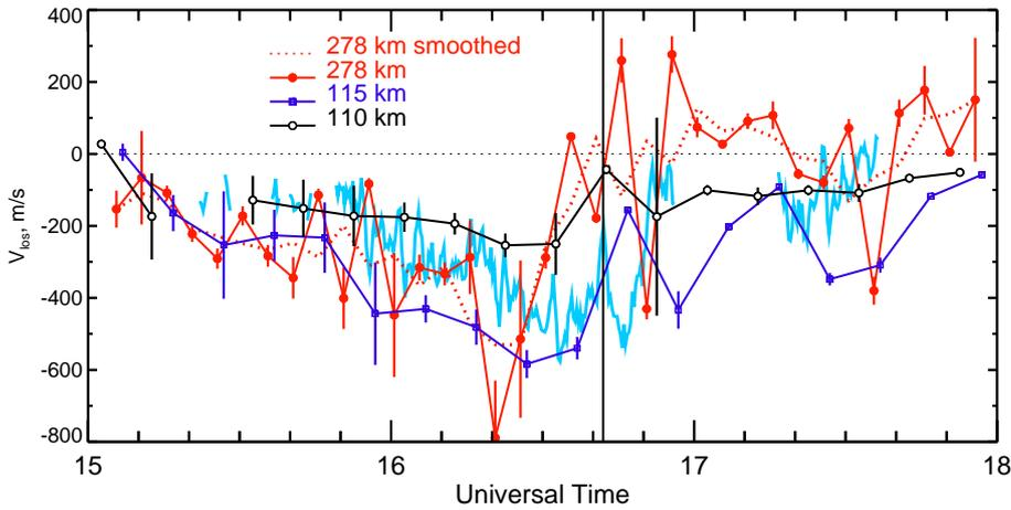
**Fig. 3.** Comparison between the components resolved along the STARE beam 4 direction. The red, dark blue, and black lines show the EISCAT ion drift velocity component at 278, 115, and 110 km, respectively. The light blue line is the Doppler velocity measured by the STARE radar in the radar cell corresponding to a range of 855 km. The vertical line shows the time of density enhancement at 16:42 UT from Fig. 2a.
