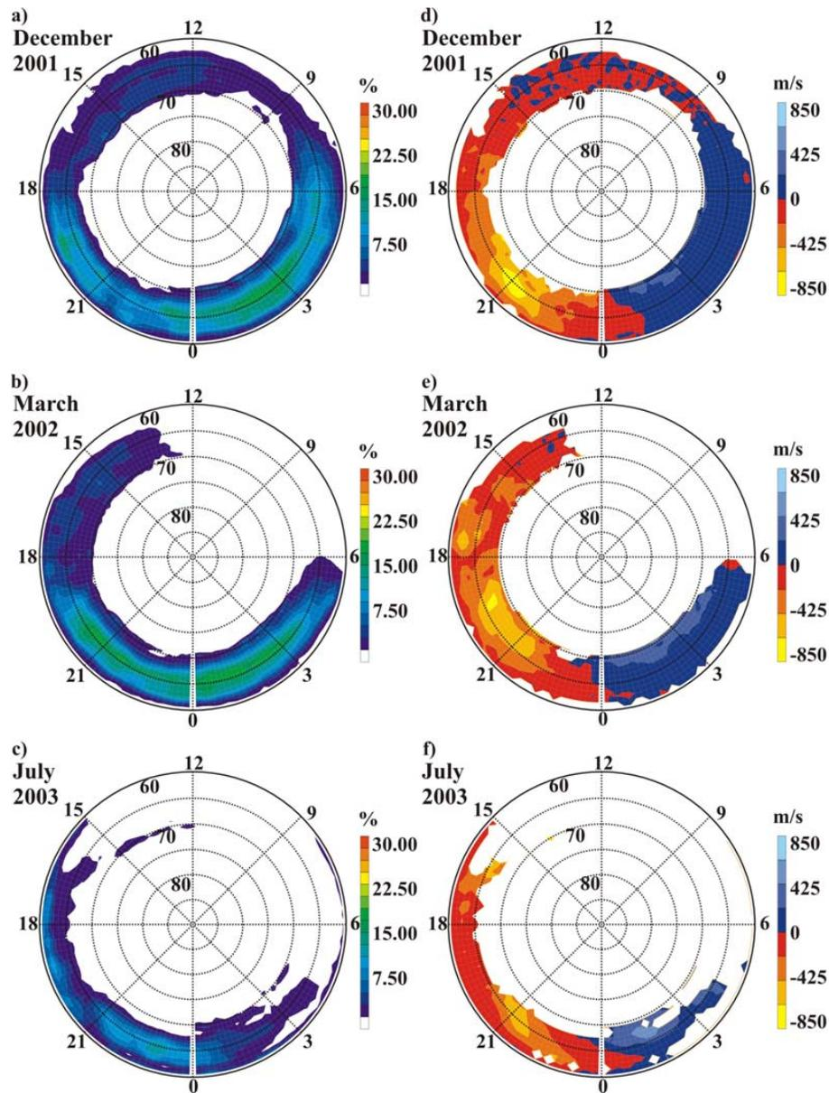
**Fig. 2.** King Salmon echo occurrence rate and averaged line-of-sight velocity for winter (December 2001, panels (a) and (d)), equinox (March 2002, panels (b) and (e)) and summer (July 2003, panels (c) and (f)) in magnetic latitude – magnetic local time coordinates. Only data in beams 0-5 were considered.
