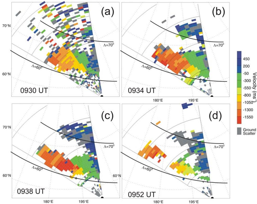
**Fig. 10.** King Salmon 1-min velocity maps illustrating the onset of very high-velocity echoes roughly along the L-shell directions between ~09:34 and 09:38 UT. These echoes correspond to the extremely fast flow identified in Fig. 8c. The transition from the very high velocities to the background ones is seen well in the central beams as a sharp velocity magnitude decrease.
