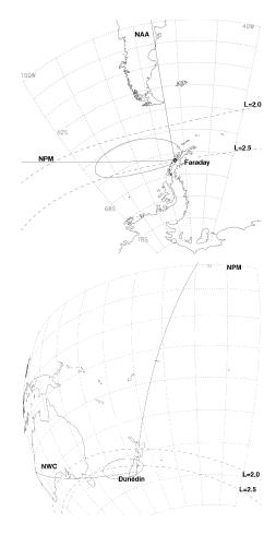
**Fig. 2.** Maps showing the VLF paths for Trimpi observations undertaken in this study, along with the L=2.0 and L=2.5 contours at 100 km altitude. An ellipse marks the WEP modified ionospheric region used in our calculations. Top Panel: the region around the Antarctic Peninsula and the location of Faraday Station. Bottom Panel: the region around New Zealand and the location of Dunedin.
