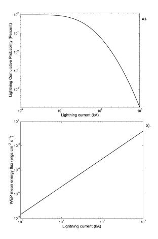
**Fig. 6.** (Top panel) Cumulative statistical distribution for CG lightning return stroke peak currents. (Lower panel) Magnitude of the WEP mean energy precipitation flux expected from a given lightning return stroke peak current.
