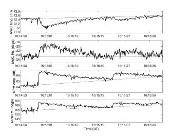
**Fig. 4.** An example of a fairly large Trimpi event observed on transmissions from NWC and NPM at Dunedin on 1 November 2003. The time resolution is 0.4 s. The unperturbed behaviour of the signals is indicated by the long dashed lines.
