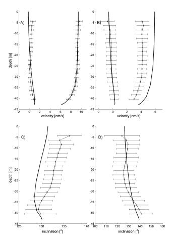
**Fig. 13.** Tidal ellipse's vertical structures at the J station for M2: (A) – major and minor semi-axis, (C) – inclination angle, and K1: (B) – major and minor semi-axis, (D) – inclination angle tidal constituents. Stars represent observed values, error bars mark the observation error, and the bold line represents model predictions.
