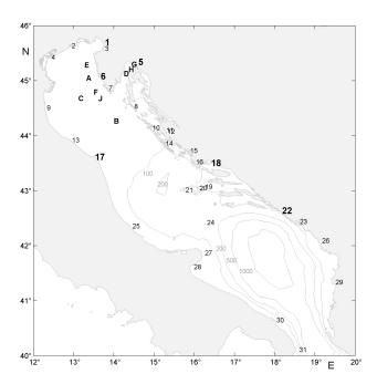
**Fig. 1.** Location map with bathymetry of the Adriatic Sea. Gauge stations based on literature values are represented with numbers, those with our analysis results as large bold numbers. Locations of Aanderaa RCM-4 current meter stations are marked with letters A–H and the ADCP station with the letter J.
