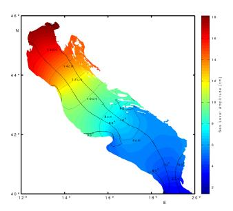
**Fig. 6.** Co-amplitude and co-phase chart for K1 tidal constituent. Amplitudes are in cm (thin dashed line with 2-cm increment) and phases (line with 10° increment) in degrees relative to 15° E.
