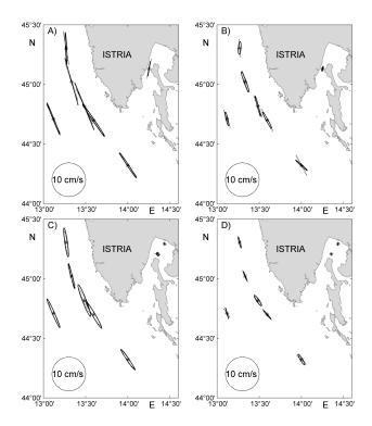
**Fig. 11.** Tidal ellipses for the M2: **(A)** surface, **(C)** bottom and K1: **(B)** surface, **(D)** bottom tidal constituents, based on observations (bold solid) and model results (dashed).
