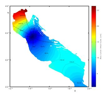
**Fig. 5.** Co-amplitude and co-phase chart for M2 tidal constituent. Amplitudes are in cm (thin dashed line with 2-cm increment) and phases (line with 30° increment) in degrees relative to 15° E.
