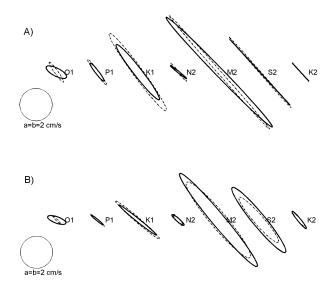
Fig. 12. Tidal ellipses for seven constituents at the J station: (A) surface -8.5 m, (B) bottom -40.5 m depth, based on observations (bold solid) and model results (dashed).
