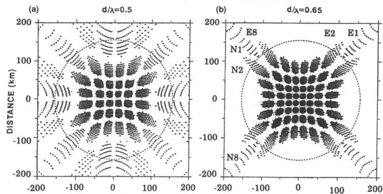
Fig. 6. The projection of a half-power width of the 64 antenna beams onto an ionospheric absorption altitude of 90 km. The patterns are shown for (a) 0.5 wavelength spacing at Zhongshan station and (b) 0.65 wavelength spacing at Ny-Ålesund station.
