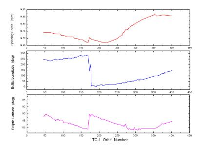
**Fig. 3.** Evolution of the TC-1 spinning speed (upper panel), the ecliptic latitude (mid panel) and ecliptic longitude (lower panel) of the spin axis of TC-1. Note that the Kepler period of TC-1 is about 27.4 h.
