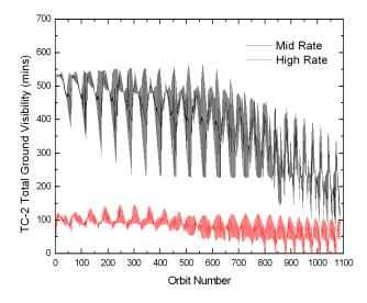
**Fig. 7.** TC-2 satellite total visibility at high and mid data dumping rates from the three ground stations.
