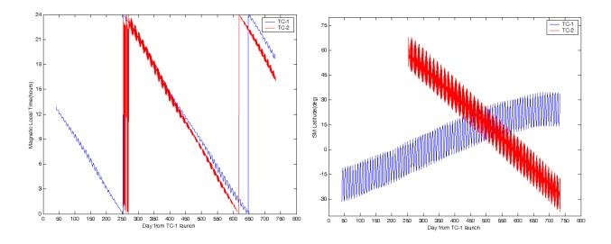
Fig. 2. Evolution of the magnetic local time (left panel) and SM latitude (right panel) of the apogee of DSP with time as predicted. The origin of the horizontal axis is the launch time of TC-1.
