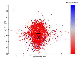
**Fig. 2.** Scatter plot of the variation of mean Doppler velocity and mean vertical signal power obtained using the VHF radar for the 68 days examined. Individual points are colour coded with the value of the surface rainfall rate measured by an ARG tipping bucket rain gauge. The centre of mass for the precipitation and no precipitation periods are identified by a plus sign and a cross, respectively.
