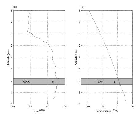
Fig. 3. Typical profiles of (a) range squared corrected signal to noise ratio,  $\tau_{\text{corr}}$ , observed by the UKMO UHF wind profiler at Aberystwyth and (b) a near simultaneous radiosonde temperature profile launched from Aberporth (approximately 50 km away from the radar site) are displayed for the 11 December 2000 at 05:30 UT. The position of the peak of the bright band identified by the automated algorithm is also displayed.
