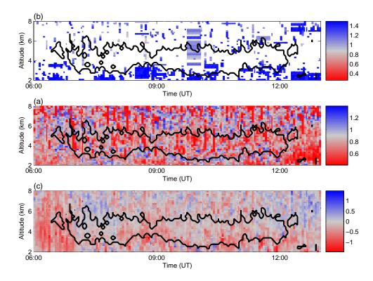
**Fig. 8.** Profiles of **(a)** precipitation signal spectral width (ms<sup>-1</sup>), **(b)** clear-air signal spectral width (ms<sup>-1</sup>), and(c) clear-air vertical velocity (ms<sup>-1</sup>) observed by the VHF wind profiler on 24 September 2000. The full line indicates the extent of precipitating cloud regions identified using simultaneous UHF wind profiler data.
