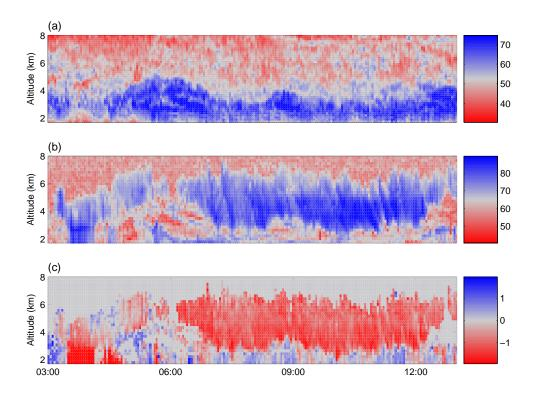
**Fig. 5.** Time-height contour plots of (a) vertical signal power (dB) observed by VHF radar, (b) the vertical range squared corrected signal to noise ratio (dB) and (c) the vertical velocity ( $ms^{-1}$ ) measured by a co-located UHF wind profiler observed on 24 September 2000. Note that the UHF data has a higher time resolution than that available in the rest of this study.
