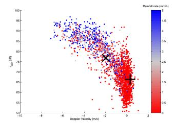
**Fig. 1.** Scatter plot of the variation of mean Doppler velocity and mean range squared corrected signal to noise ratio,  $\tau_{\text{COIT}}$ , obtained from the vertical beam of the UKMO UHF wind-profiler for the 68 days examined. Individual points are colour coded with the value of the surface rainfall rate measured by an ARG tipping bucket rain gauge. The centre of mass for the precipitation and no precipitation periods are identified by a plus sign and a cross, respectively.
