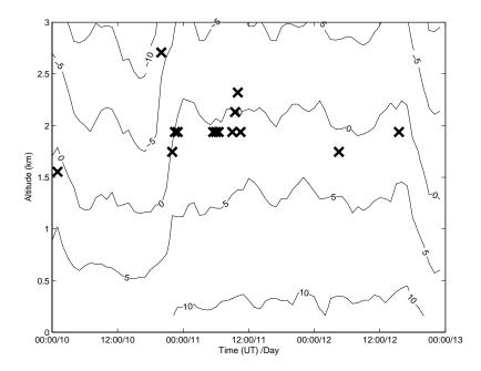
**Fig. 4.** Time-height contour plot of temperature taken from the UK Met Office mesoscale model predictions over Aberystwyth for the period 10 to 12 December 2000. Also displayed are crosses which indicate the position of the peak of the bright band identified by the bright band detection algorithm during this period.
