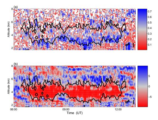
**Fig. 7.** Profiles of **(a)** vertical spectral width (ms<sup>-1</sup>) and **(b)** vertical signal power perturbation (dB) observed by the VHF wind profiler on 24 September 2000. The full line indicates the extent of precipitating cloud regions identified using simultaneous UHF wind profiler data.
