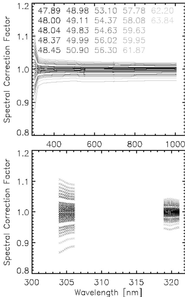
**Fig. 3.** Modelled correction factor to account for the change in SZA during the albedo measurements for 4 January 2004. The SZA corresponding to the measured downwelling irradiance spectrum is listed in the upper panel, where the complete spectral range is shown. The lower panel only shows the UVB because the spectral dependence of the correction factor is largest in the limited wavelength range.
