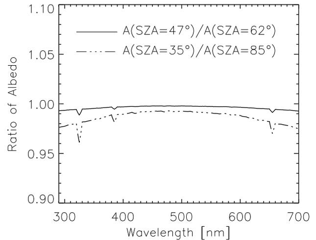
**Fig. 9.** Ratios of modelled snow albedo ( $A$ ) for different solar zenith angles. In both cases the ratio is between 0.96 and 1.0 for all wavelengths. Thus, the albedo is larger at larger SZA compared to smaller SZA. The local minima at 320, 385, and 650 nm are due to Mie scattering processes for single snow grain size radii.
