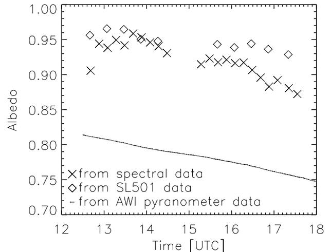
**Fig. 7.** Diurnal cycle of mean albedo on 4 January 2004 derived from different radiation sensors. For the period shown, the sky was cloud free. All sensors show a decrease in albedo the later in the day it became, thus the larger the solar zenith angle.
