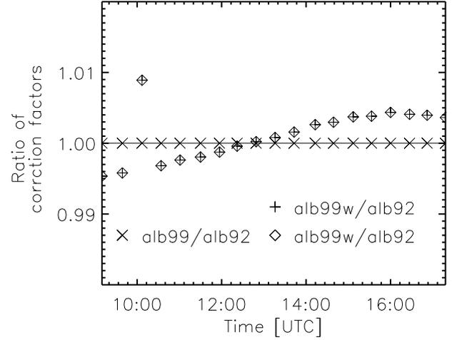
**Fig. 2.** Ratios of correction factors modelled with different input albedos for an example day. The abbreviations used in the legend represent the type of albedo and cloud input parameter for UVSPEC: alb92: albedo 0.92, no clouds; alb99: albedo 0.99, no clouds; alb92w: albedo 0.92, stratiform cloud cover; alb99w: albedo 0.99, stratiform cloud cover.
