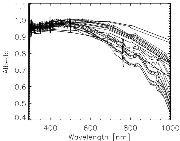
**Fig. 10.** All of these albedo spectra are measured at Neumayer with solar zenith angles between  $48^\circ$  and  $49^\circ$  on different days and times (morning and/or afternoon). The difference in albedo spectra is lowest at 400 nm with 0.08 and it becomes larger the larger the wavelength.
