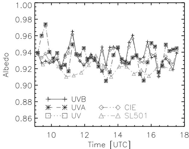
**Fig. 8.** Diurnal cycle of different integral albedo values measured on 2 January 2004. The sky was covered by stratiform clouds. A dependence of albedo on time (thus SZA) cannot be observed for this day.
