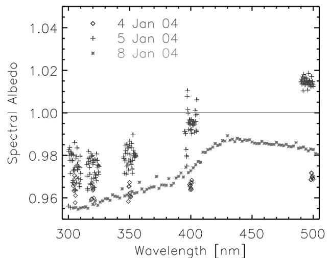
**Fig. 5.** Same as Fig. 4, but the wavelength range is limited (295 to 505 nm). On 5 January 2004, the albedo is larger than unity with 1.015 at 500 nm, which is an effect of direct incidence of solar radiation.
