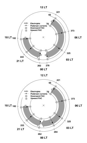
**Fig. 4.** (a) Schematic of the directly driven currents in the auroral oval between dawn and dusk, used in the model to describe the growth phase of a substorm just before the EP onset. (b) Same as Fig. 4a but for conditions just after substorm EP onset.
