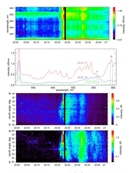
**Fig. 5.** Spectrograph data at Apatity: (a) evolution of spectrum averaged in  $0^{\circ}$ -18° North zenith angles (the region marked by "1" in Fig. 1); (b) spectra at several moments; (c) north-south keogram in "A" emission band (655.7–656.2 nm, mainly Doppler-shifted H $\alpha$ ); (d) north-south keogram in "B" emission band (659.3–659.8 nm, N<sub>2</sub>1PG).
