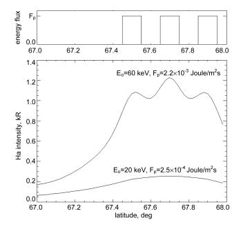
**Fig. 11.** H $\alpha$  luminosity as a function of latitude, stimulated by three regions of precipitated protons. Top panel is a latitudinal section of precipitation structure. Bottom panel presents the spatial structures of the column-integrated luminosity for two cases of proton precipitation parameters.
