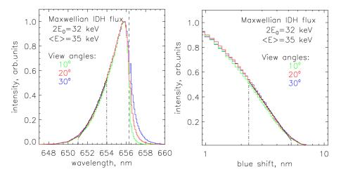
**Fig. 8.** Simulated H $\alpha$  profiles for view angle relative to the magnetic field line direction: green  $-10^\circ$ ; red  $-20^\circ$ ; blue  $-30^\circ$ . Black solid line is the least-squares fit of Eq. (1), dash-dotted line marks the fit range, dashed line is a position of non-shifted H $\alpha$  line. (a) full profiles; (b) blue-shifted wing in log-linear coordinates.
