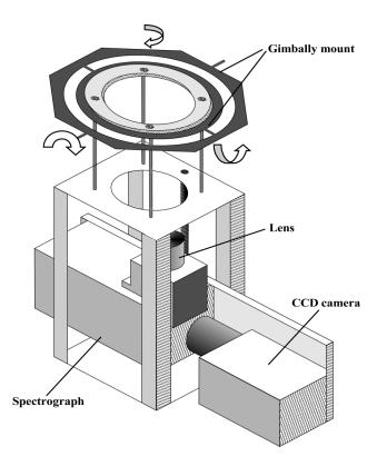
Fig. 2. Schematic of the spectrograph SpectraPro 306 with CCD camera IpentaMax.
