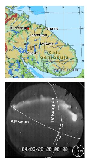
Fig. 1. Geometry of observations: (a) observation points; (b) fields of view for optical devices.
