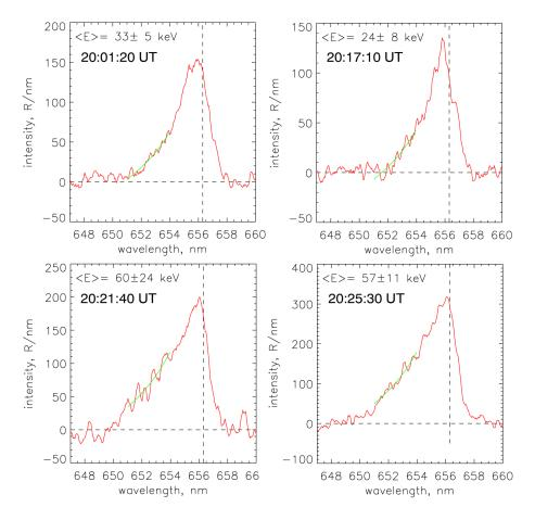
Fig. 9. Examples of observed H $\alpha$  profiles (red lines) and the least-squares fit of the blue wing by Eq. (1) (green lines).  $\langle E \rangle$  is an estimated average energy of precipitated protons. Dashed lines mark a position of non-shifted H $\alpha$  line and zero intensity level.
