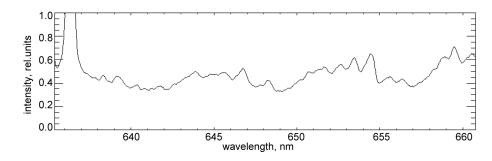
Fig. 6. Average spectrum of electron excited lines in the spectral range of 636.0–661.0 nm.
