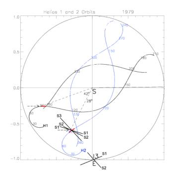
**Fig. 1.** The trajectories of Helios-1 (black trace) and Helios-2 during 1979, shown in a system with a fixed Sun-Earth line. The near-Earth spacecraft ISEE-3 is marked *I*3. The ecliptic projections of the shock fronts at both locations are also indicated.
