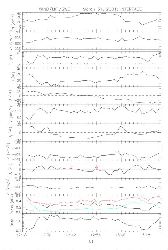
**Fig. 9.** The interface between ejecta 1 and 2. The panels show from top to bottom the proton density, bulk speed and temperature, (pairwise) components of field and flow in principal axes coordinates (i, j, k); the pressures (blue: magnetic field, black: plasma (electrons plus protons) and red: their sum), and the proton beta.
