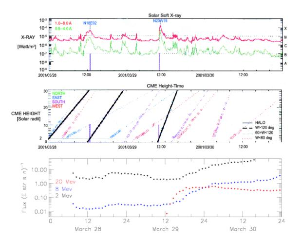
Fig. 8. Solar observations (top panels). Bottom panel: LEMT/EPACT measurements of high energy proton fluxes. A dispersional injection is seen starting at  $\sim$ 12:00 UT, 29 March in the highest energy panel.
