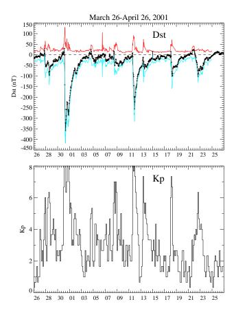
**Fig. 10.**  $K_p$  and  $D_{st}$  measurements for 26 March– 26 April 2001. The effect of the  $\alpha$ -particles in calculating the magnetopause currents (top red trace) has not been taken into account. For further details, see text.
