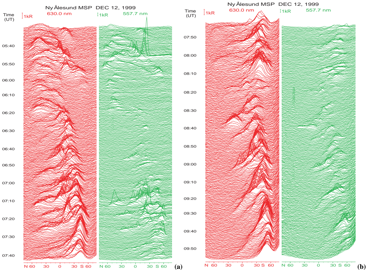
Fig. 17. MSP observations from Ny Ålesund during the intervals (a) 05:30–07:40 UT and (b) 07:40–09:55 UT. Left and right columns show stacked plots of line of sight intensity vs. zenith angle for the wavelength channels at 630.0 and 557.7 nm, respectively. Same format as in Fig. 3.
