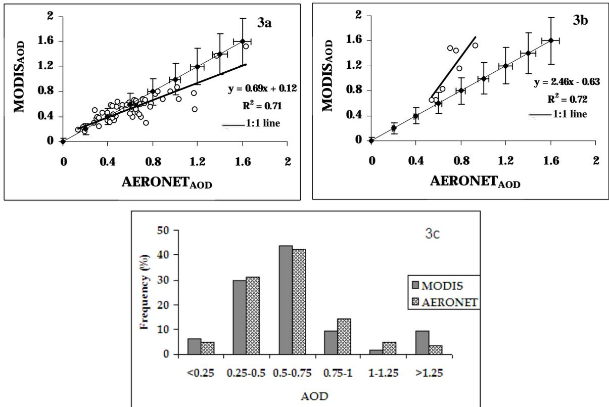
**Fig. 3.** Scatter plot between AOD derived from MODIS and AERONET in 2004 during (a) non-dust loading period and (b) dust-loading period and (c) frequency distribution of AOD derived from AERONET and MODIS. The error bars in Figs. 3a and b indicate the range of MODIS expected accuracy ( $\pm 0.05 \pm 0.2\tau_a$ ) from the 1:1 line (along Y-axis) and the uncertainty of AERONET measurements (along X-axis).
