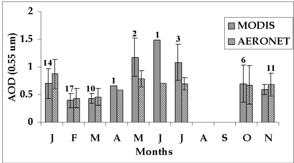
**Fig. 2.** Monthly averaged AOD at 0.55 μm wavelength over Kanpur during the year 2004 retrieved from MODIS and AERONET. The error bars represent the standard deviation of AOD for that month. Numbers above the histogram of MODIS derived AOD represent the number of data points for the respective month.
