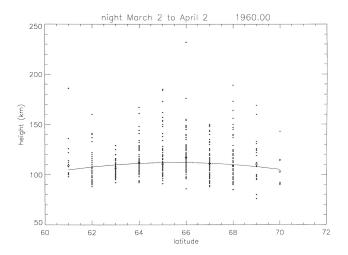
**Fig. 9.** Distribution of the height of the peak emission of 5577 Å [OI] emission as a function of dipole latitude for only the nighttime data (solar depression angle  $>18^{\circ}$  from the 1960 observations. The line is a second order polynomial least squares fit and the diamonds are median values.
