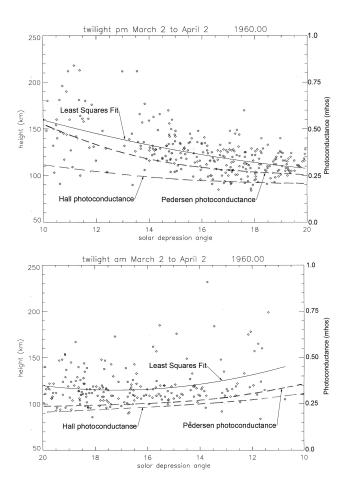
**Fig. 5.** (a) Same as Fig. 4a, except for all eight days in March and April of 1960. A second order polynomial least squares fit to the data is shown along with the conductance as a function of solar depression angle. (b) Same as Fig. 5a, except for morning twilights.
