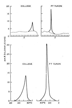
**Fig. 2.** Raw data from two simultaneous photometer scans from College and Fort Yukon (upper panel). The background brightness is removed by subtracting the dotted line from the data. The peaks in the remaining data are used to triangulate on the location of maximum brightness (lower panel).
