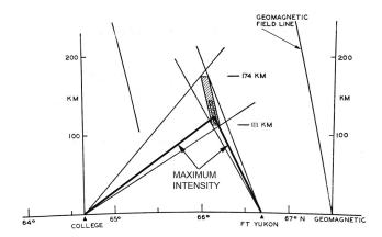
**Fig. 3.** Showing the method of locating the maximum 5577 Å [OI] intensity as triangulated from the two stations in the magnetic meridian.
