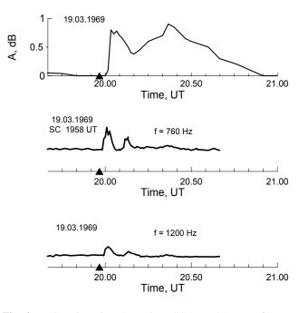
**Fig. 2a.** Cosmic noise absorption (SCA) and bursts of VLFemission observed on 19 March 1969. Planetary magnetic activity preceding the SC event is low ( $K_p=1+$ ). The time of the SC is indicated by the black triangle.
