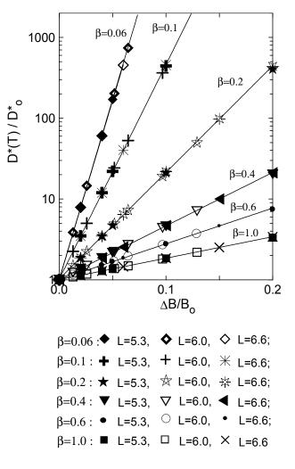
**Fig. 6.** Magnitude of relative change of diffusion coefficient  $D^*(T)/D^*(t_0)$  as a function of  $\Delta B/B_0$  obtained for different values of parameter  $\beta$ .
