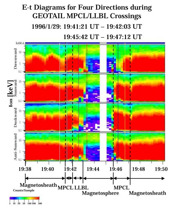
**Fig. 5.** Ion energy-time spectrograms for four directions (dawnward, sunward, duskward and antisunward directions) of two MPCLs and LLBL crossings during the interval from 19:38:00 UT to 19:50:00 UT on 29 January 1996. The ion population from 5.0 counts/sample to 500 counts/sample is shown with the lower color bar. Two MPCL crossings are bracketed by broken lines.
