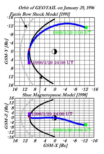
**Fig. 2.** The orbit of GEOTAIL on 29 January 1996 projected onto the GSM-X and -Y (upper) and GSM-X and -Z (lower) planes. The start (00:00 UT) and end (24:00 UT) points of the trajectory are marked by green and purple solid boxes, respectively. The locations where GEOTAIL crossed the MPCL/LLBL are marked by red points. The gray and black curves show the model bow shock (Farris et al., 1991) and magnetopause (Shue et al., 1998), respectively.
