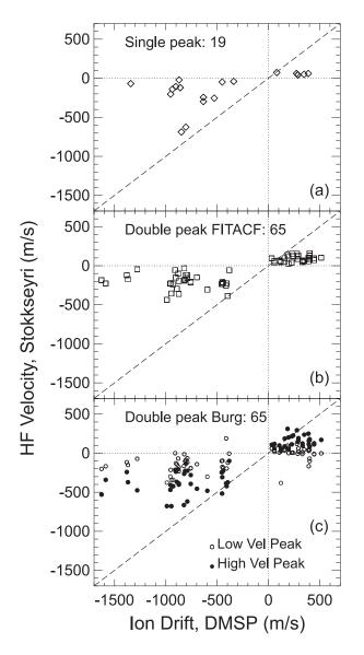
**Fig. 5.** A comparison of the Stokkseyri 1-o-s velocity (FITACF) and DMSP cross-track ion drift for 22 events. Panels (**a**) and (**b**) correspond to the cases of single- and double-peaked HF echoes. Panel (**c**) shows velocities of low- (open circles) and high- (filled circles) shifted components of the double-peaked echoes as given by the Burg spectrum analysis.
