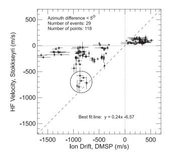
**Fig. 4.** The line-of-sight Stokkseyri velocity versus DMSP ion drift when the deviation between the radar and satellite directions of measurements were less than  $5^{\circ}$  and the differences in time were less than 2 min.
